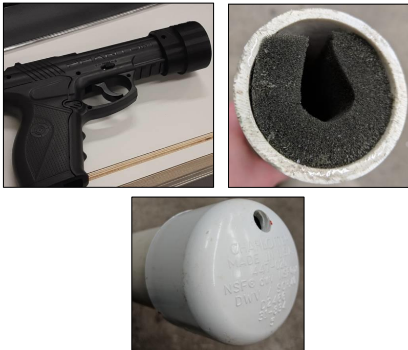
Fig. 22: Muffer adapter piece (left), foam added inside muffer (right), PVC end cap (bottom)
